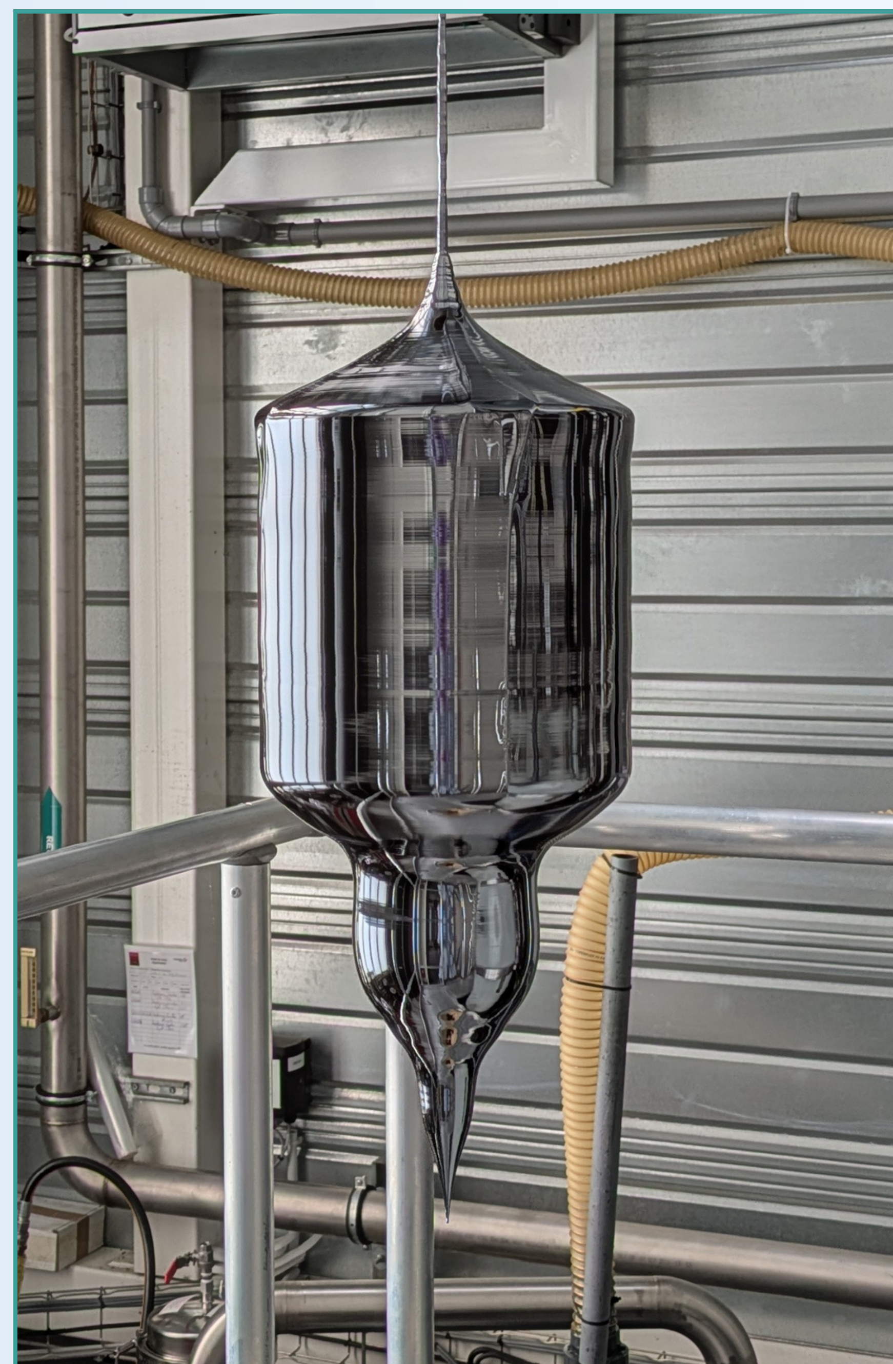
Cz ingot unloading: (left) 11% recycled silicon/89% EG ; (right) 12% recycled silicon/88% EG
