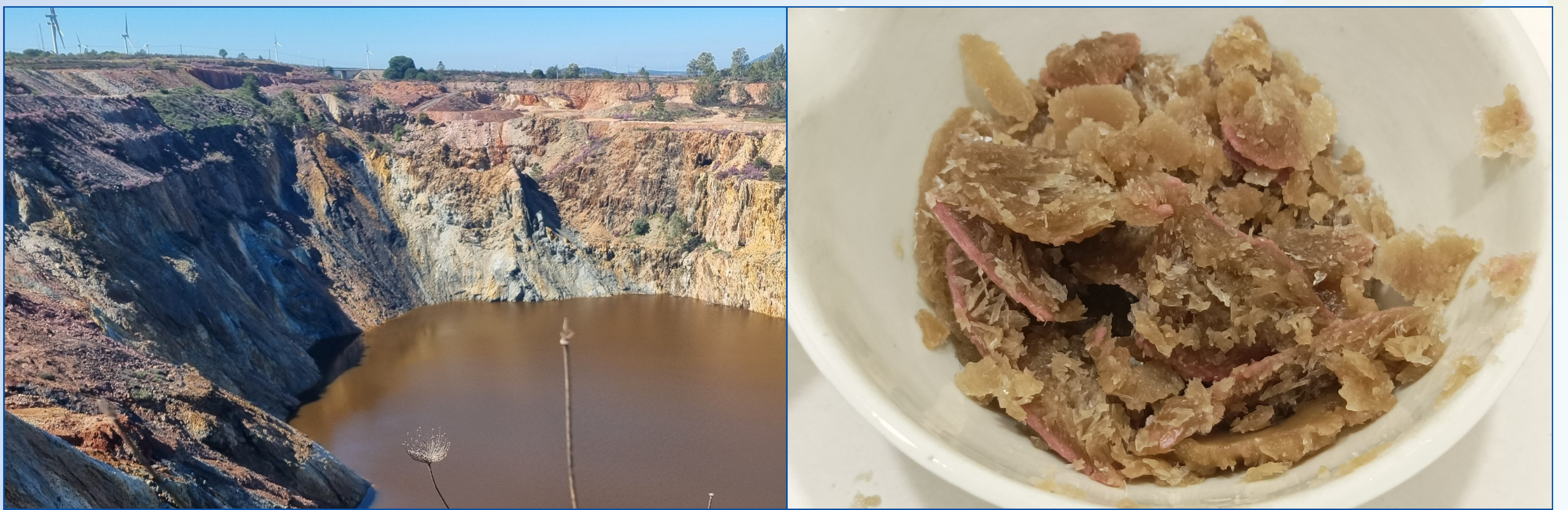
Left: Acid waste water at Tharsis Mining Right: Cobalt and Nickel crystals obtained from the treatment
