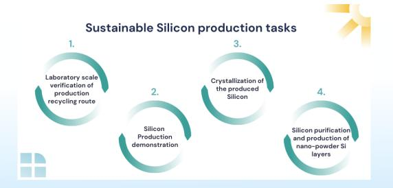
In order to reach this goal, NTNU will work on demonstrating a circular process to produce high purity silicon through aluminothermic reduction of quartz fines, followed by refining of the produced metal utilizing kerf, originating from the cutting wire during wafering of Silicon and representing a loss of more than 40 % of silicon during the process.
