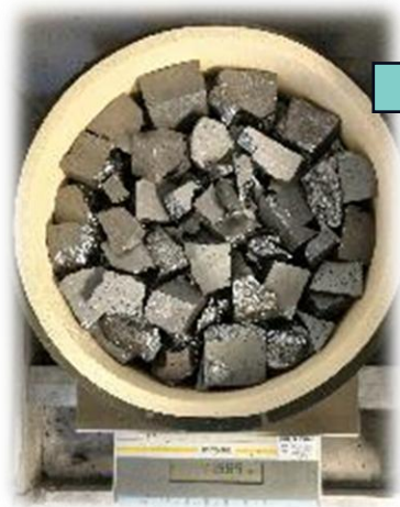
Si metal obtained in slag refining (98.91 % Si)
