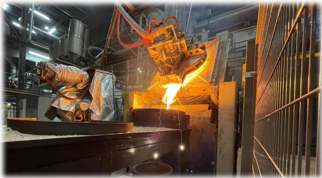
400kg (600 kW induction furnace) => 97,79% Si
