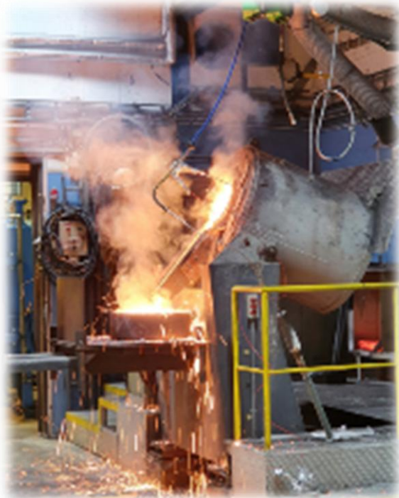
50kg (225 kW induction furnace) => 98,91% Si
