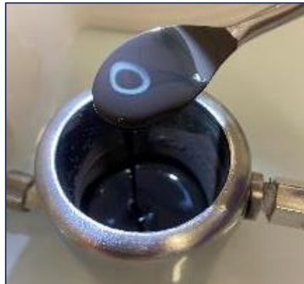
Incorporation and dispersion easy to do ( D_{100} < 20 \mu\text{m} )
