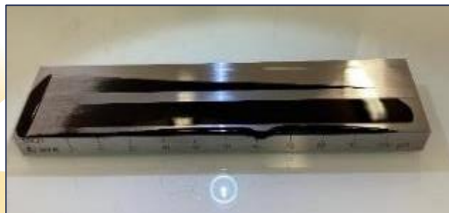
Incorporation and dispersion easy to do ( D_{100} < 20 \mu\text{m} )
