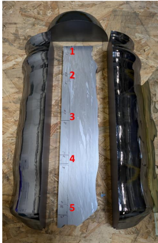
Figure 16: Recycled silicon" ingot from crystal pulling – Five GDMS samples along ingot height
