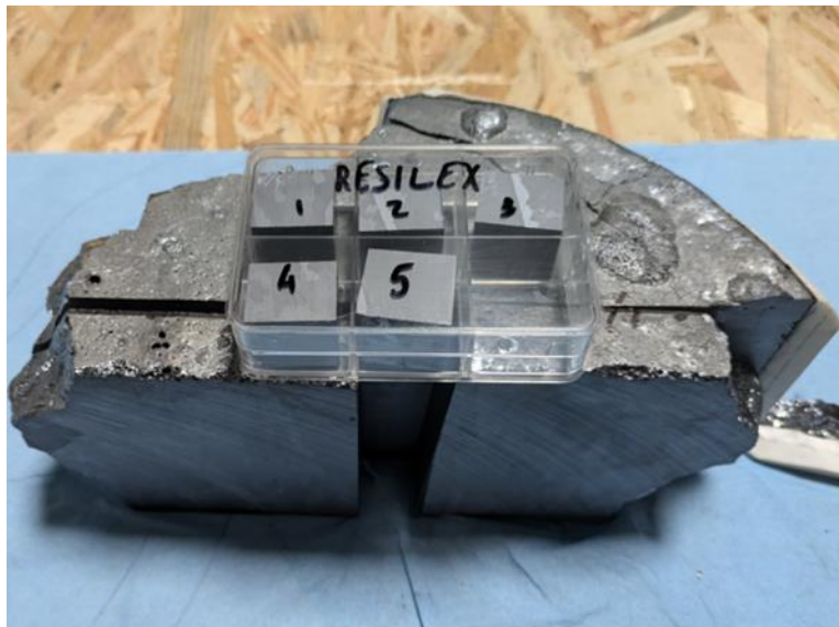
Figure 7: "Recycled silicon" ingot after additional directional solidification - Five GDMS samples.
