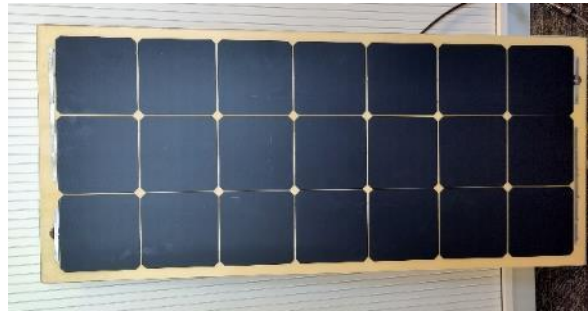
Figure 14 Lightweight module with a wood backsheet
