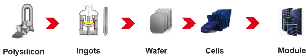
Figure 1: Value chain of a silicon PV module
